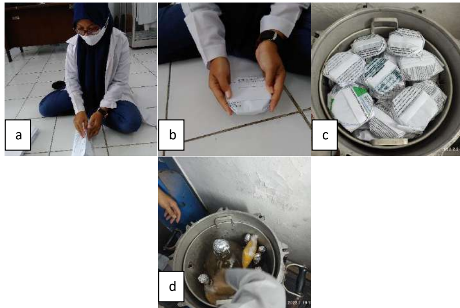
Figure 5. 1 Sterilization of Tools and Materials, (a) Wrapping petri dishes, (b) Petri dishes that have been wrapped, (c) Equipment to be sterilized, (d) Media to be sterilized. (Source: Personal documentation).
