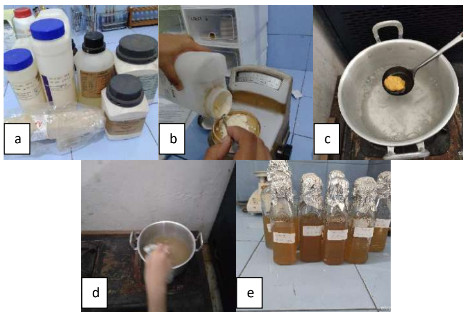
Figure 5. 4 Making King's B Media, (a) King's B media materials, (b) Weighing King's B media materials, (c) Putting media materials into distilled
